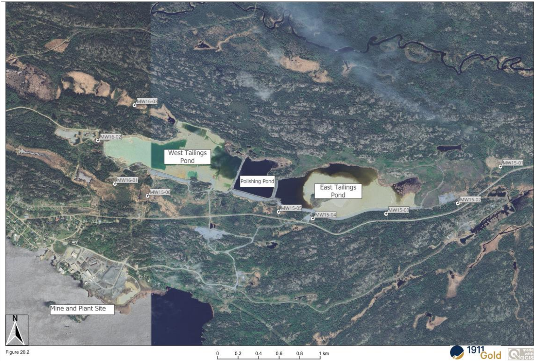
Figure 20.2 Aerial view of the mine, plant site, and TMA with monitoring well locations
