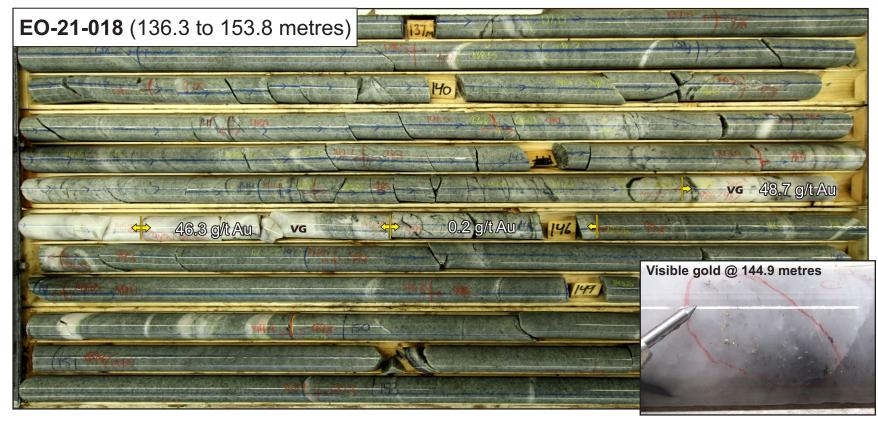
Figure 2: Shear vein with high-grade gold in drillhole EO-21-018; inset shows disseminated visible gold (silver-grey minerals are interpreted to be Bi-Te phases, which are common in gold ores in the Rice Lake district). Shear vein is localized along a pronounced change in alteration intensity and veining in the Gunnar porphyry.
